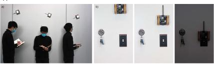
To demonstrate the function and extendibility of the Climbot, we present two simple applications. Figure a) shows a light carried by the Climbot that is dynamic and can follow the user indoors. Figure b) shows another example where the robot goes to a switch to turn a lamp off on-demand. Collaborative jobs can potentially be done by synchronizing multiple bots.
